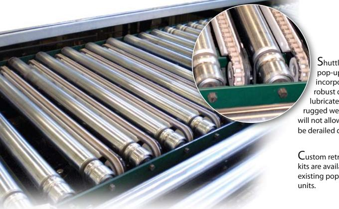
Shuttleworth's pop-up transfer incorporates a robust design of nonlubricated chain and rugged wear strip which will not allow the chain to be derailed during transfers.
